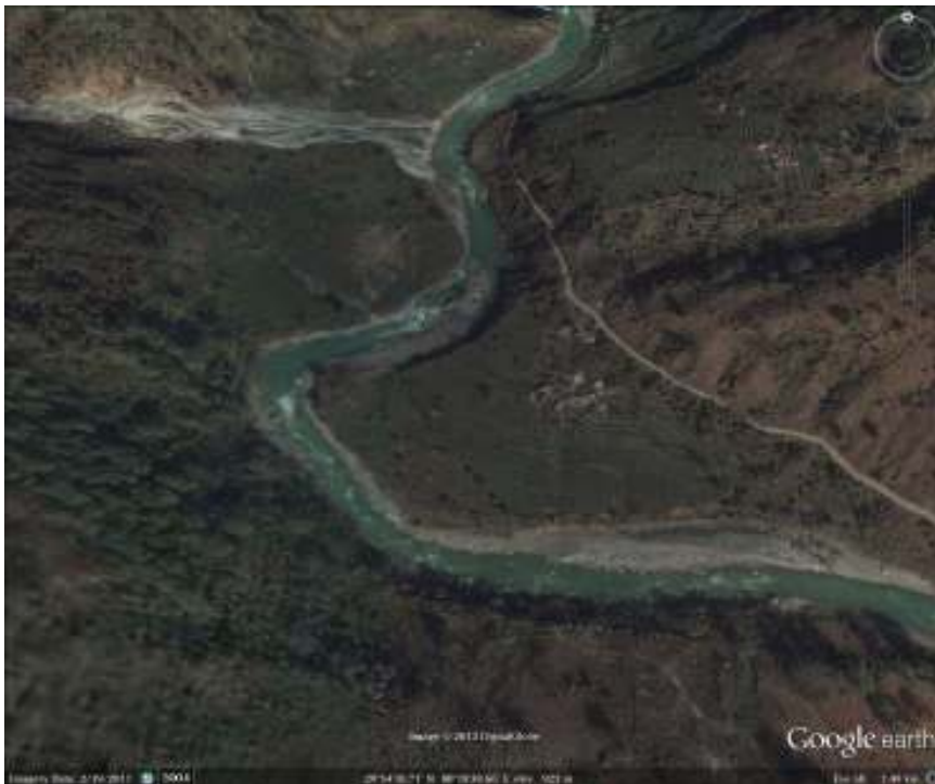
Figure 6: A Google earth image, from 2004, showing Talla Mori village, to the center right, located at a safe distance of over 200 meters from the Gori river. Here not only has the river changed course but has created a new flood plain on the left (the true right bank).
